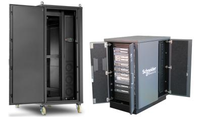
Figure 1 Examples of micro data centers
